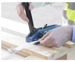
Release the tension handle. Insert the upper strap into the slot of the housing & the windlass.
