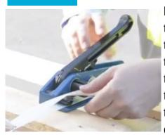
hand & depress the handle. Place the strap under the gripper so that it touches the housing with the right hand edge.
