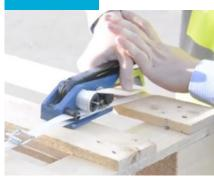
Depress the tension handle to cut the strap.
